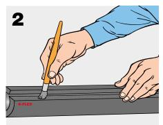
Cut the insert along its length and glue into place.
