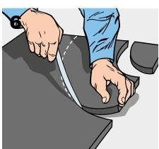
Using a compass, mark the out-line of the internal radius on the K-FLEX® sheeting, using the corner of the square marked out on the insulating material as the axis.
