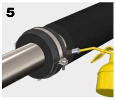
Glue support edges with K-FLEX® glue and join the two halves on the pipes.
