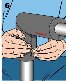
Carefully glue the edges of the elbow section to the straight tubes to be positioned either side.
