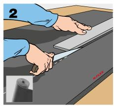
Position the uncovered edge at the starting point (a). Pull the backing paper off gradually, pressing the material down as you go. Use K-FLEX® glue to join the edges together. In the example given, for the best results we recommend first to insulate the lower surface of the conduit, then the side walls and lastly the top. This will prevent the penetration of humidity.
