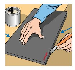
sheet around the tubing, ensuring that the seam does not overlap that of the underlying insulation.
