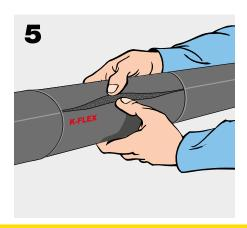
Once the glue has dried, reseal the tube, pressing the edges firmly together.
