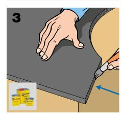
Position the throughsection shape on the piping and join the glued edges.
