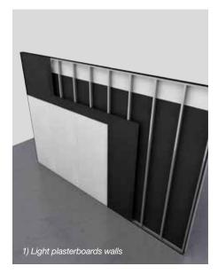
K-FLEX® glue to GK/GV and to the metallic surface. Put the GK/GV on the metallic panel. A 50mm overlap between two consecutive panels will give better results avoiding acoustic bridges. For thicker material (over 4kg/m² weight) use additionally a mechanical fixing with screws or pins every 50cm.
