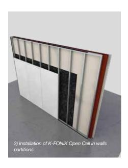
panel. For thicker material (over 30mm thick) use additionally a mechanical fixing with screws or pins every 50cm. Open Cell can be glued also on GK/GV substrate Apply K-FLEX® glue to K-FONIK OPEN CELL and to the GK/GV surface. Put the K-FONIK OPEN CELL on the panel. For thicker material (over 30mm thick) use additionally a mechanical fixing with screws or pins every 50cm.
