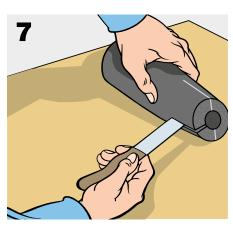
Glue the edges of the cut-outs together so that the diameter of the tubing reduces.
