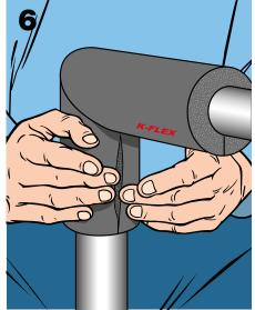
If the straight sections have already been glued into place, the right-angled section will have to be accurately measured to fit.
