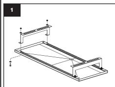
Position the tray hangers to match the width span of the wall bracket. Secure with fixings.
