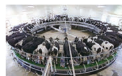
"Rotary parlour" that milks 50 cows. It takes about 10 minutes to rotate once.
