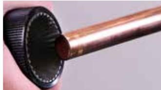
2. Deburr and remove all external sharp edges
