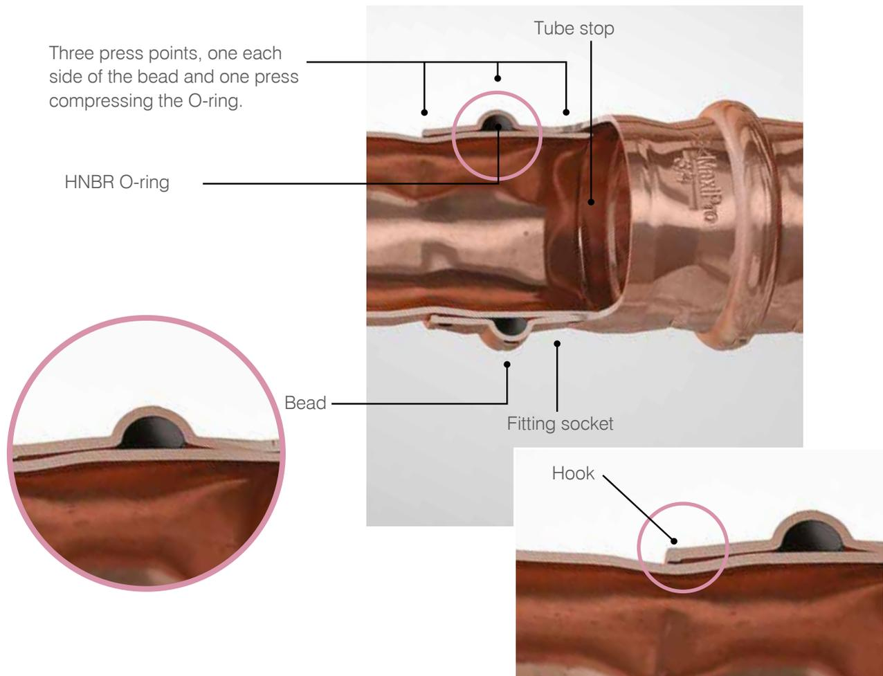
On fittings 1/2" and upwards, a hook ensures that the high pressure performance achieved by >B< MaxiPro fittings is maintained.
