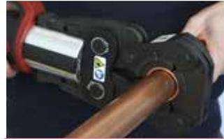
3. Complete the joint with the press tool
