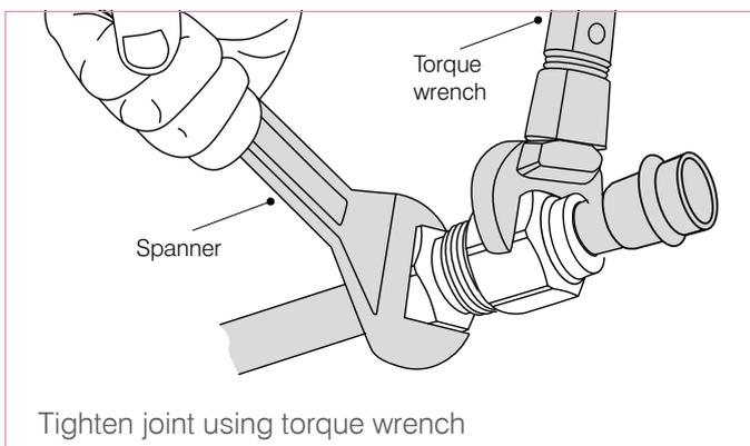
Fully tighten using spanner and torque wrench to the torque values set out in table 9. **Do not over tighten.**
